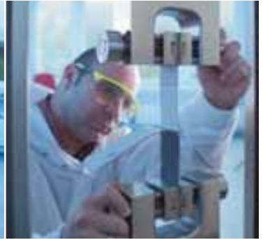
Peel testing with welded plastic specimens.
