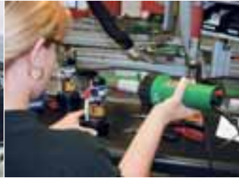
Shrinking a solder sleeve with TRIAC PID.
